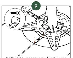
Use the 5x16 wooden screw to attach the cable clips to the table top. Secure the cables on each side of the connection of the interconnecting cables.
