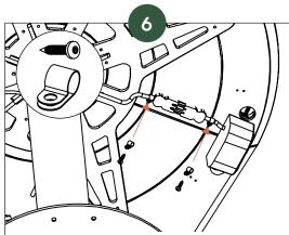
Use the 5x16 wooden screw to attach the cable clips to the table top. Secure the cables on each side of the connection. Reapeat on both charger connection.
