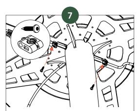
Use the 5x35 wooden screw to attach the cord relief to the table top through the star disk. Secure the cables going out from the trunk. Reapeat on both chargers.
