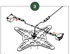
Connect the phase chargers to the interconnecting cables. NOTE: the next following steps needs to be done after completing the assembly of your Seamless Table.
