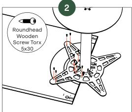
Use the 5x30 wooden screw to attach the table top to the seamless table lower trunk.
