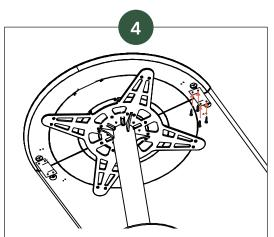
Use the screws that are included in the phase charger to attach the plastic plate to the table tops. Repeat on both sides.
