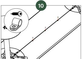
Use the 5x16 wooden screw to attach the cable clips to the table top. Secure the long interconnecting cable along the table top all the way to the next lower trunk.
