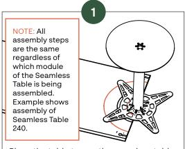
Place the table top on the seamless table lower trunk. Make sure to align the holes of the star disk with the slots in the table top.
