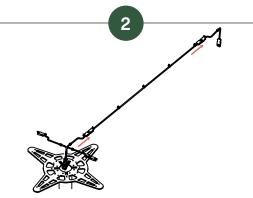
Take the middle one of the three interconnecting cables that is already connected in one end and connect the other end to the long interconnecting cable. Connect the other side of that cable to the last interconnecting cable 500mm.
