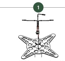
Connect three interconnecting cable 500 mm to the adaptor block and place it in to the seamless table lower trunk. Connect your starter cable if you have that comming from the trunk.
