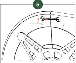
To tighten the connection armatures and close the gap between the table tops, use an allen key. NOTE: Allen key not included.
