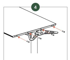
Place the wood dowels in the holes in the table top.
