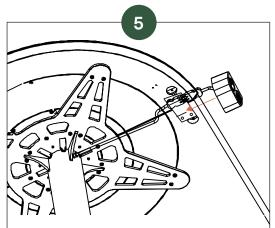
Slide the phase charger on to the plastic plate until it clicks in place. Repeat on both chargers.
