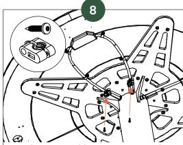
Use the 5x35 wodden screws to attach the cord relief to the table top. Attach the cabels close to where the cable exits and enters the trunk.
