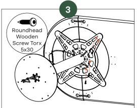
Attach the table top from the seamless table module using the 5x30 wooden screw in the points of the star disk and in all holes of the inner circle.
